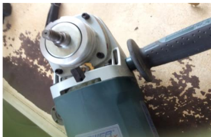
Figure 3.6: Operational testing of the grinding machine with the produced carbon brush.
