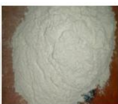
Figure2. Particulate snail shell filler
