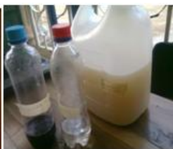
Figure3. The unsaturated polyester, accelerator and catalyst used.
